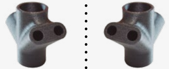
Mirror printing with 2 extruders
